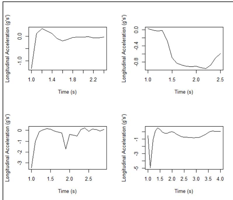
**Figure 15. A sample of acceleration profiles during crashes.**
