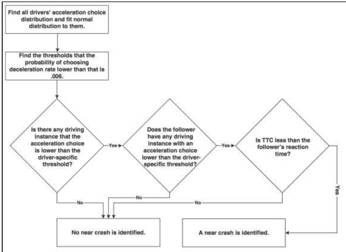
Figure 7. Method 1 as recommended by Talebpour et al. [12].
