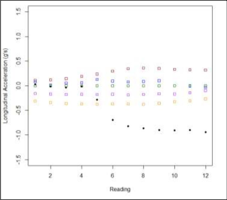
Figure 17. Crash comparison (black dots) with baseline readings.
