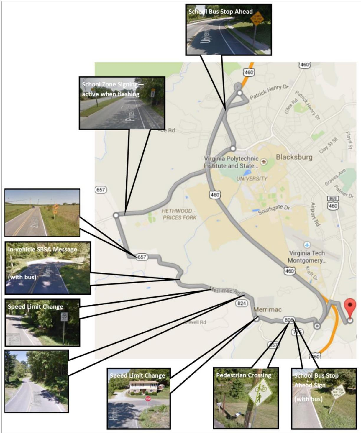
Figure 10. Map of the test route showing the types and locations of key events.
