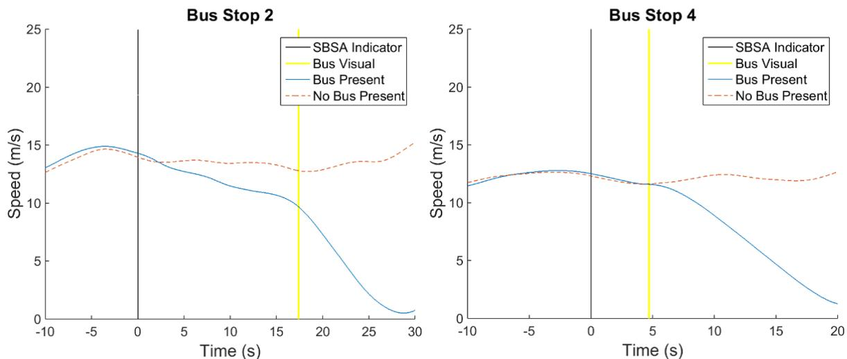
**Figure 21. Comparison of vehicle speeds approaching the bus stops indicated via in-vehicle message. (Bus Stop 2 on left, Bus Stop 3 on right).**
