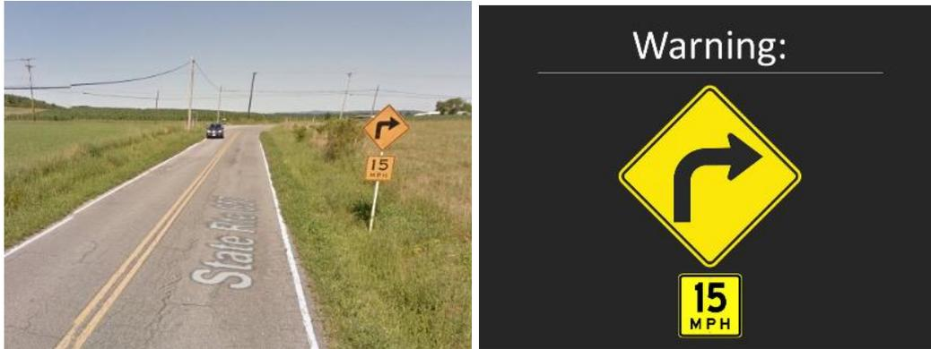
**Figure 17. Location of (a) curve advisory warning and (b) in-vehicle display of curve advisory speed sign.**
