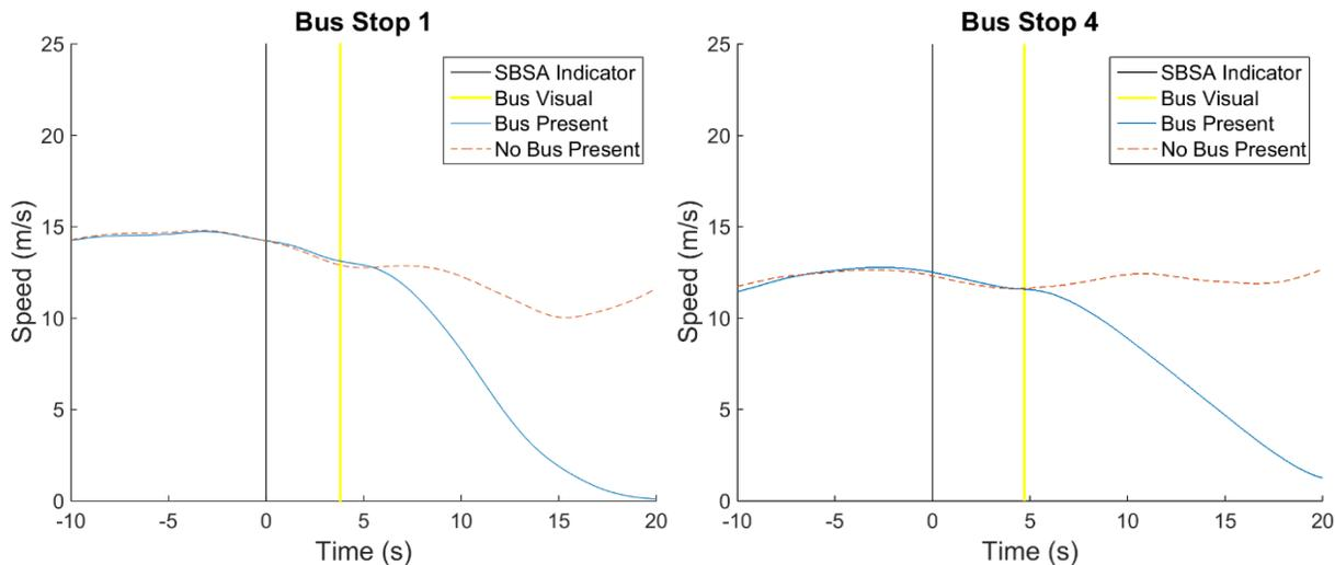
Figure 20. Comparison of vehicle speeds approaching the bus stops indicated via roadside sign. (Bus Stop 1 on left, Bus Stop 4 on right).
