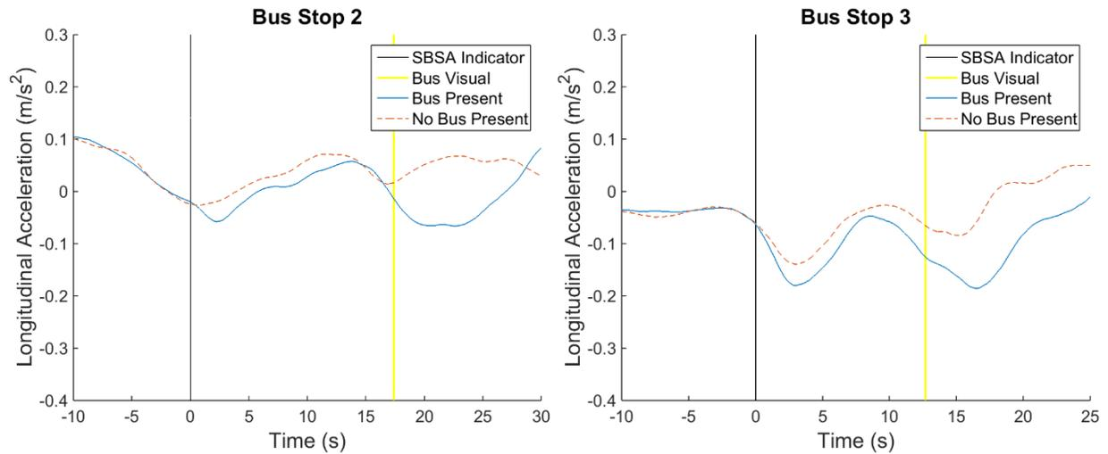
**Figure 23. Comparison of driver longitudinal accelerations approaching the bus stops indicated via in-vehicle message. (Bus Stop 2 on left, Bus Stop 3 on right).**
