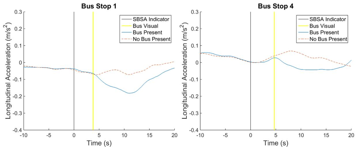
**Figure 22. Comparison of vehicle longitudinal accelerations approaching the bus stops indicated via roadside sign. (Bus Stop 1 on left, Bus Stop 4 on right).**
