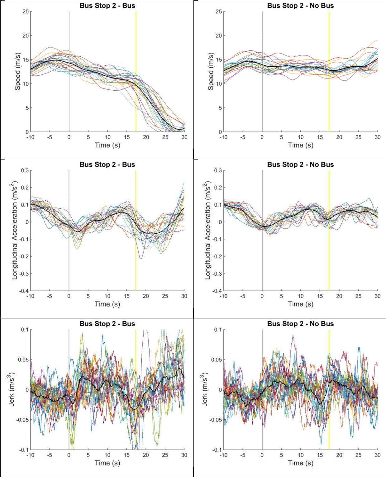
Figure A.2. Bus Stop 2 – in-vehicle SBAS.
