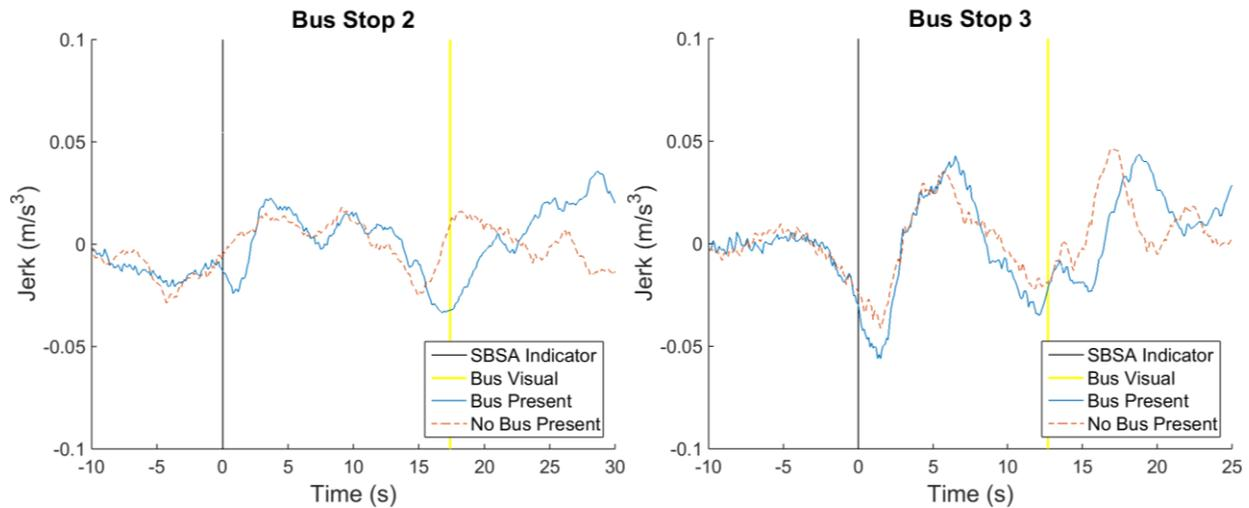
**Figure 25. Comparison of vehicle jerk when approaching the bus stops indicated via in-vehicle message. (Bus Stop 2 on left, Bus Stop 3 on right).**
