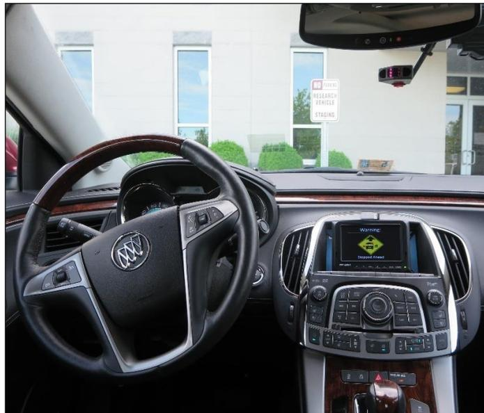
**Figure 5. View of the test vehicle message display system.**
