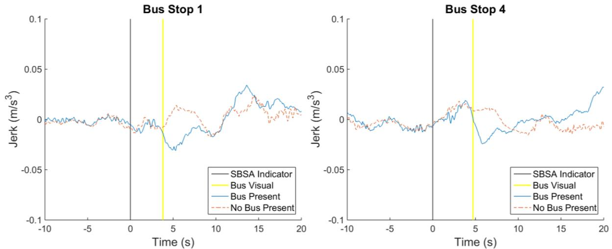
**Figure 24. Comparison of driver jerk approaching the bus stops indicated via roadside sign. (Bus Stop 1 on left, Bus Stop 4 on right)**
