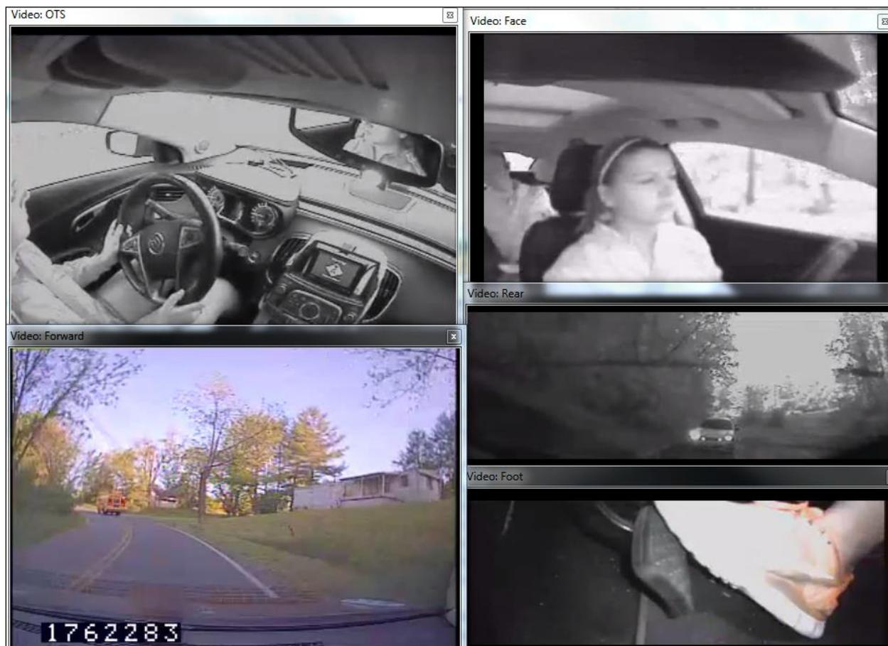
**Figure 6.** Camera views on the test vehicle (over the shoulder camera [top left], forward-facing camera [bottom left], face camera [top right], rear-facing camera [middle right], and foot/brake pedal camera [bottom right]).
