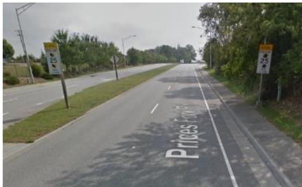
**Figure 18. School zone signs (active when flashing).**
