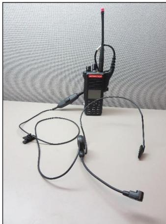
**Figure 8. Image of radio communicators.**
