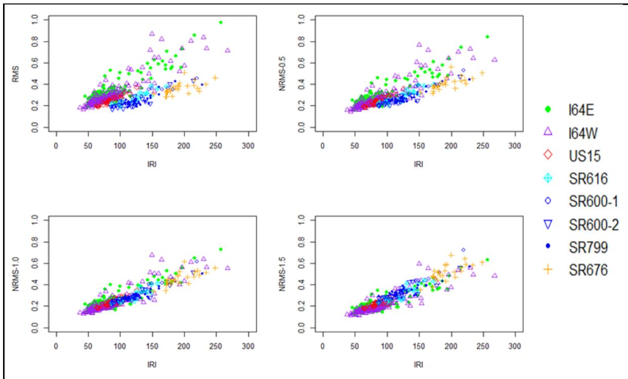
**Figure 9. Scatter plots of IRI vs. RMS/NRMS acceleration.**
