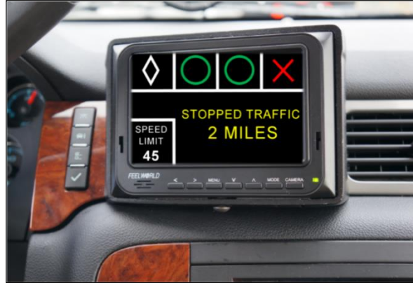
Figure 1. In-Vehicle Device (IVD).
